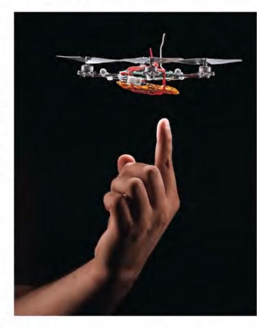
This "micro air vehicle" with four rotors, made by KMel Robotics in Pennsylvania, can fly in swarms with its mates. The drones navigate autonomously, without a pilot. UAVs," says Richard Scudder, who runs a University of Dayton laboratory that tests prototypes. One serious accident, Scudder points out, such as a drone striking a child playing in her backyard, could set the industry back years. "If we screw the pooch with this technology now," he says, "it's going to be a real mess."
